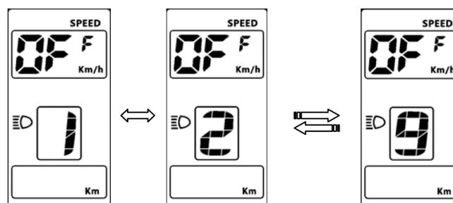
**8.4 Wheel diameter** : The location of speed displays symbol **Wd**, press **UP/DOWN** button rotate display the symbol **16/18/20/22/24/26/700C/28/29**, value represents the diameter of the wheel (inch). Wrong value for wheel diameter will cause speed&mileage abnormal.
