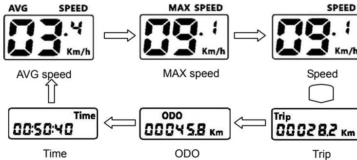
Speed mode switch& Mileage mode switch
