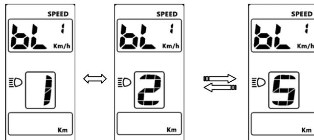
**8.3 Auto off time** : The location of speed displays symbol **OFF**, press **UP/DOWN** button to change the value from **1** to **9**, the number represent delay time (minutes) before display shutdown automatically, default value is 5 minutes.
