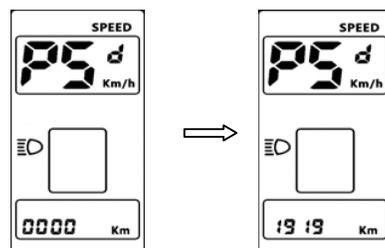
**8.7 Speed limit set** : The location of speed displays symbol **SPL**, the location of mileage displays speed limit value, the default value is **25km/h**. Press **UP/DOWN** buttons to modify the value, the value can be set from 10 to 45km/h. Press **POWER** button to confirm when you finish the adjustment.
