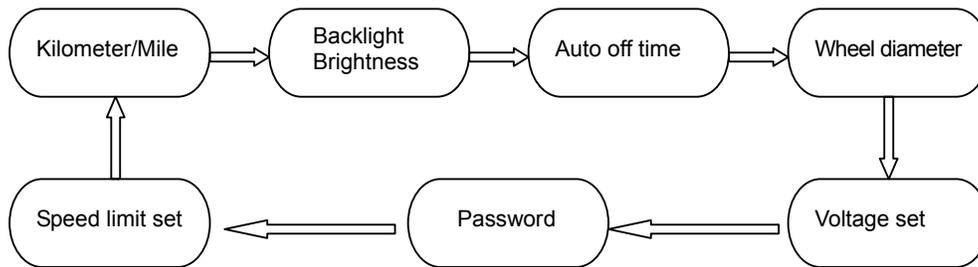
**8.1 Kilometer / Mile** : The location of speed displays symbol **S7**, press **UP/DOWN** button rotate display the symbol **km/h / MPH (Km / Mile)**
